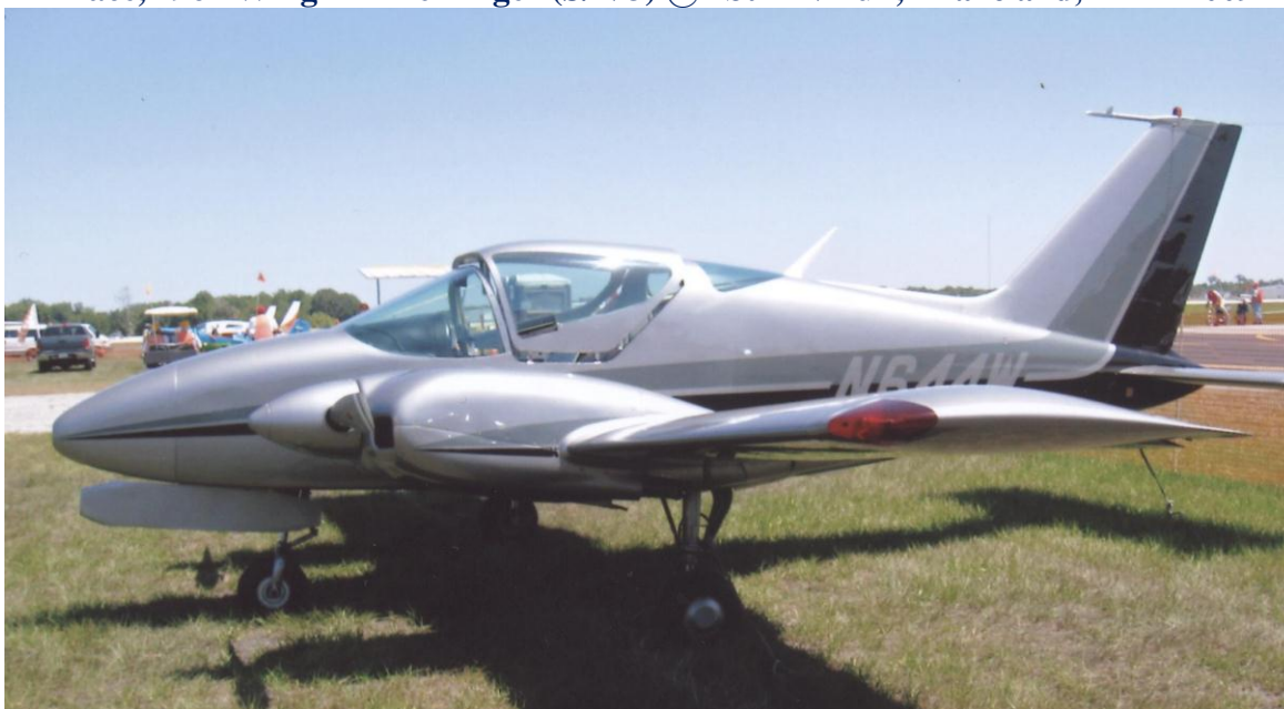
Two 160 hp Lyc. Engines, MGW = 3050 Lbs., 212 MPH Cruise, 12 were built Wikipedia Image
