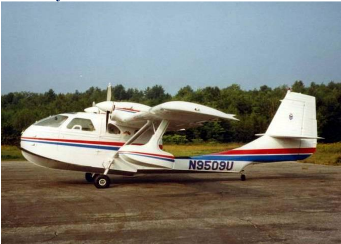
Lyc IO-360-B1D Eng. @ 180HP ea. ~ 23 Produced (1965-1987) N9509U is S/N 021 Hobie Tomlinson Image
